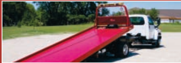
2006 GMC C5500, 26,000 GVW, 300HP Duramax, auto trans, loaded cab, with a 22' Vulcan steel carrier, fixed rails, bed-painted red, (8) add chain locks, strappless wheel lift, 48" tool box, Sock #T4284.
