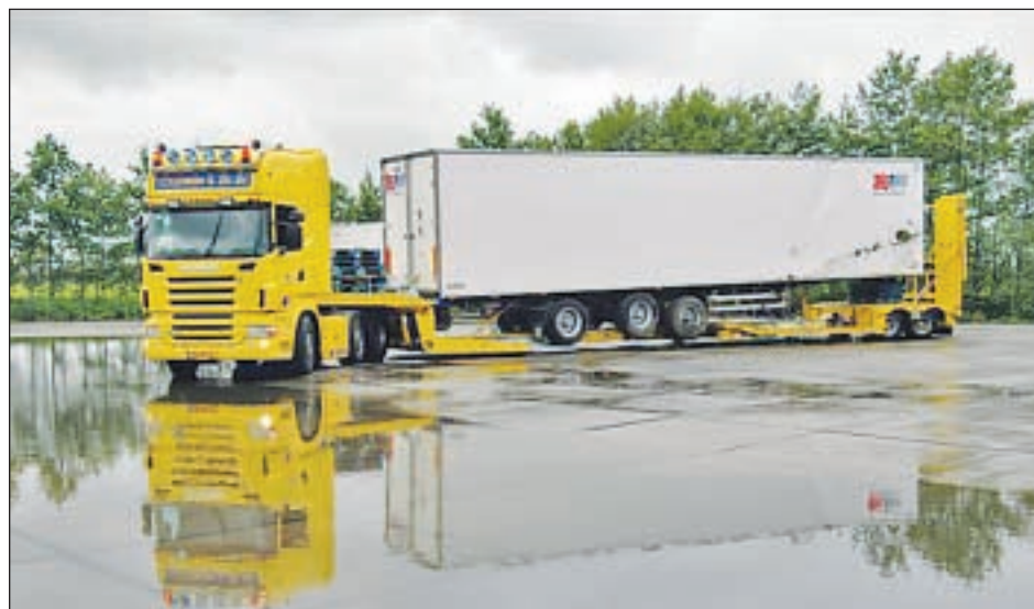
A new low loader built by GS of Meppel for Collewijn Towing and Recovery of Groenekan in Holland. The trailer will transport three vans, two tractors, or a truck, bus, or trailer on the 12-meter-long deck between the wheels. In Europe the height restriction is four meters, but these units have a permit for 4.30 meters and can transport all trucks and buses that are four meters high. Sliding-axle trailers are too high for transport in Europe.
