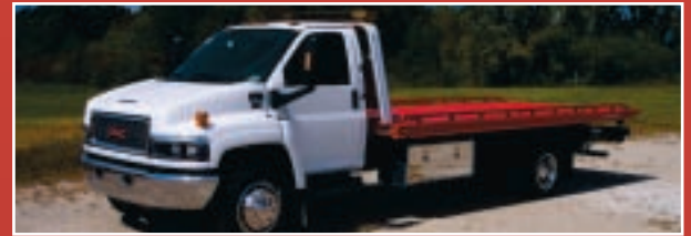
2006 GMC C5500, Duramax, Auto Loaded Cab, 26,000 GVW, with a 21' Vulcan Steel Carrier 102" Wide, Remove rails, Strapless Wheel Lift, Stock #T4290
