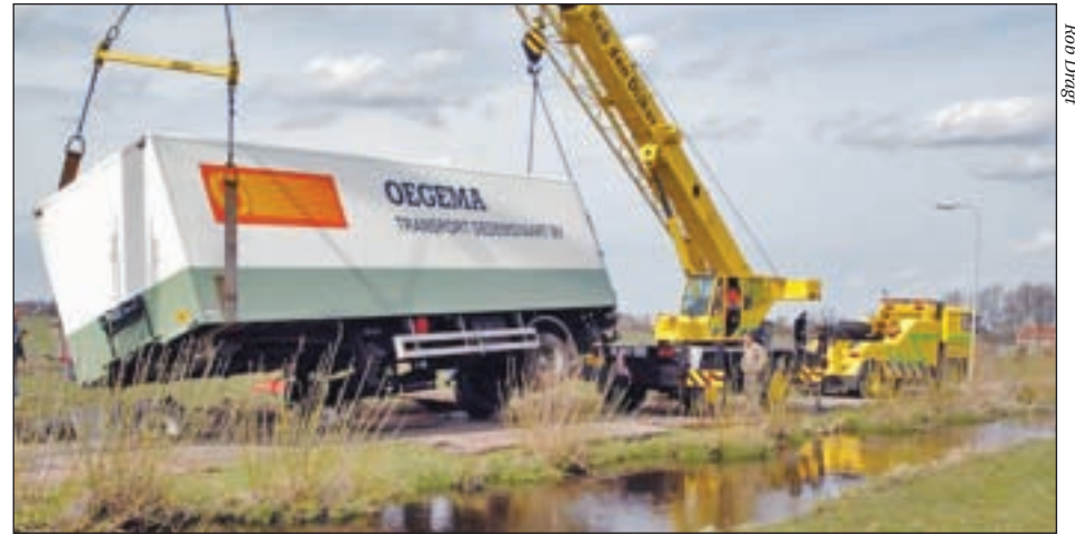
In Europe, one or two mobile cranes are often used for recoveries
