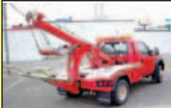
2006 Ford F450 XLT 4X4, diesel, auto, Jerr-Dan MPL40 self-loader with dual 8K lb winches, extendable boom, tow sling, in cab controls, Stk#N2589. Multifunctional unit
