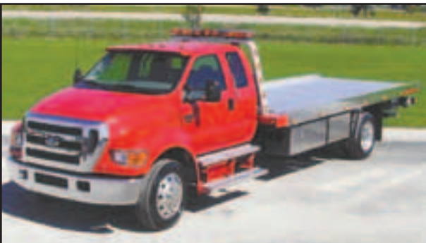
FORD F650 SUPER CAB Featuring 260 hp, automatic transmission, Chevron 21' aluminum car carrier.
