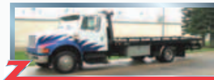
2000 IH 4700 w/Vulcan 19' Steel Carrier. DT466 - 195 HP Diesel, Auto, Axle Ratio 3:42, GVW 25,500#. MX7000 Light Bar, Stationary Cab Guard, Close Cross Members, Removable Side Rails, 2 - 48" Tool Boxes. #8184
