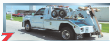
2003 Chev K30 4x4 w/Century 301. 8100 Gas, Auto., GVW 12,000#. 12 Volt Portable Air Compressor, Jet Strobe Light Bar, Self Loading Dollies. #7751
