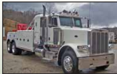
New Peterbilt 388, Glider Kit, White with Red Boom, 36" Sleeper with Window in Rear, 475 CAT, 13 Speed Transmission, 40K Air Trac Suspension, Double Framed, Leather Seats, Navigation System, Tilt & Telescopic Wheel, AM/FM CD, CB, PW, PL, Winch Brakes, 10 Alum. Wheels, Vortex Breathers, Texas Bumper, 4 Air Horns. Equipped with a New Century 9055 Alum. Wrecker Body, LED Strobe Light Bar, New Style Tubular Pylon, Power Touch Wireless Remote, 2 Speed Winches, Comes with Standard Towing Attachments. Call For Price
