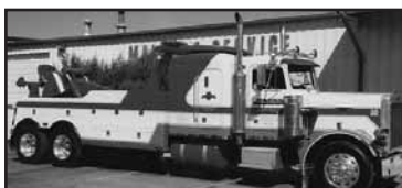
1982 Peterbilt 359, 400 Cummins, 15 speed, engine brake, double steel frame, air-ride, 58,000 miles on engine rebuild, new clutch and transmission, 96 Century 5030/T, 30,000lb. underlift, remote control. Call 505-884-1025
