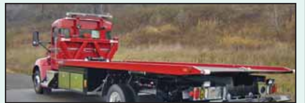
2010 PETERBILT 335, 33K GVW, 300 HP PACCAR/CUMMINS, ALLISON AUTO. CENTURY 15 SERIES STEEL CARRIER WITH A SP 8000 SIDE PULLER
