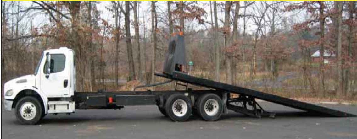
2004 FREIGHTLINER M2-106; CAT 3126 6 CYLINDER (300HP) DIESEL ENGINE; FULLER ROAD-RANGER 9 SPEED (8+LO) TRANSMISSION; TANDEM AXLE; AIR RIDE SUSPENSION; POWER STEERING; AIR BRAKES; A/C; 275/80R22.5 TIRES; 53,880 Lb GVW (13,880 FRONT, 40,000 Lb REAR); LEDWELL 28' WOOD ROLLBACK; REAR STABILIZERS;
