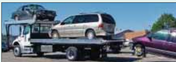
CENTURY 10 SERIES 22', 3 CAR CARRIER. INSTALLED ON A 2009 IHC 4400 WITH EXTENDED CAB SLEEPER PACKAGE. 33,000# G.V.W. MAXXFORCE DT 300 HP MOTOR, ALLISON AUTO
