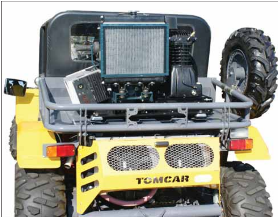
TomCar has a generator aboard
