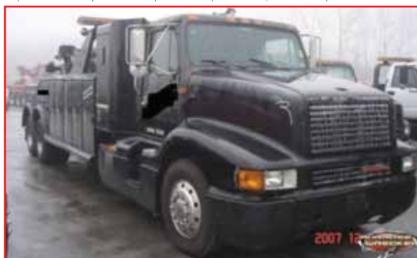
1988 INTERNATIONAL 7200 S MODEL , 315hp Cummins, 9 spd trans., 122K miles, ac, spring susp., 292" WB, drivers air susp. seat, Jerr-Dan 500-280, 25 ton boom, 2-25,000lb. winches, 3 stage underlift, 4 pr. axle forks, air winch free spools, hyd. rear spades, Code 3 light bar, air and elec. hookups, 1997 model body, stk#535491
