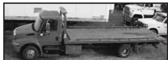
2002 International 4300 DT466, Auto Tans., A/C, Power Windows, Locks, Jer-Dan 21' 10,000lb Steel Bed, 8,000 Winch, 3,000lb Wheel Lift
