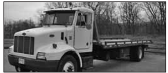
1995 PETERBILT 330, 10 Ton 28' Steel 3 Car Rollback, CAT Diesel, 33,000 GVW, Air Brakes, 2-Deck Winches.
